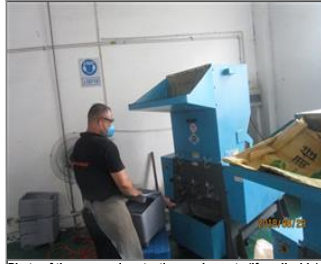
Photo of the personal protection equipments (if applicable) Ear-plugs mask and goggles used by material crushing and mixing worker.JPG
